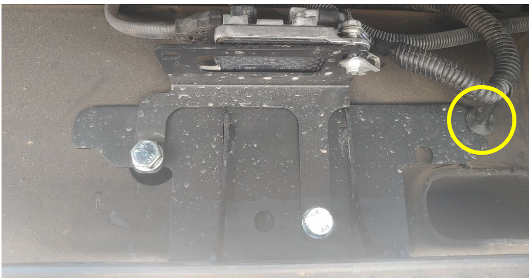
Figure 14- Compressor Bracket Installation 2, Diesel
