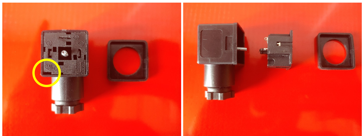
Figure 24- Connector / Housing Separation
