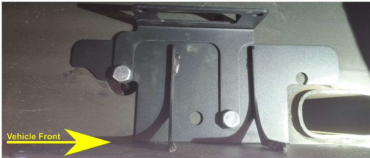
Figure 9- Compressor Bracket Installation, Outside Frame Rail
