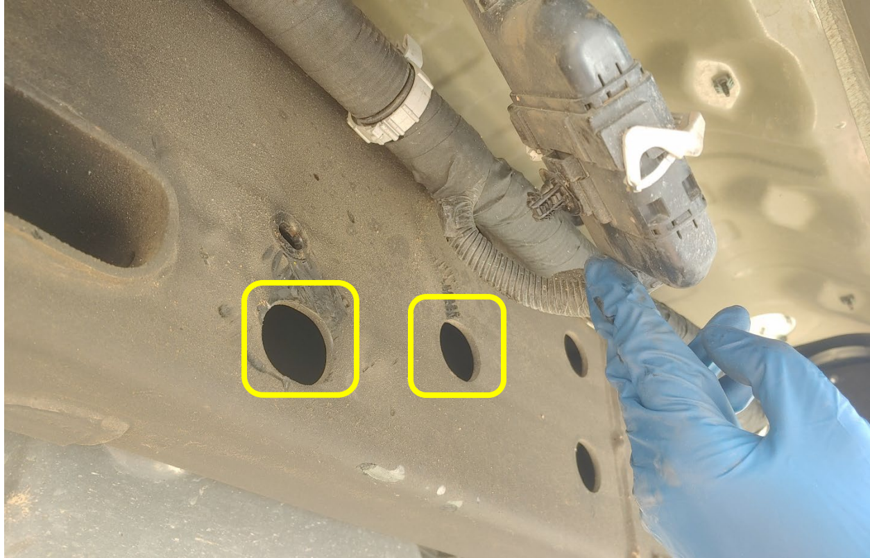
Figure 16- Tank Frontmost Bracket, Mounting Point
