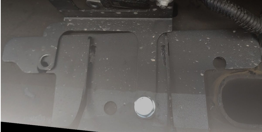
Figure 13- Compressor Bracket Installation 1, Diesel
