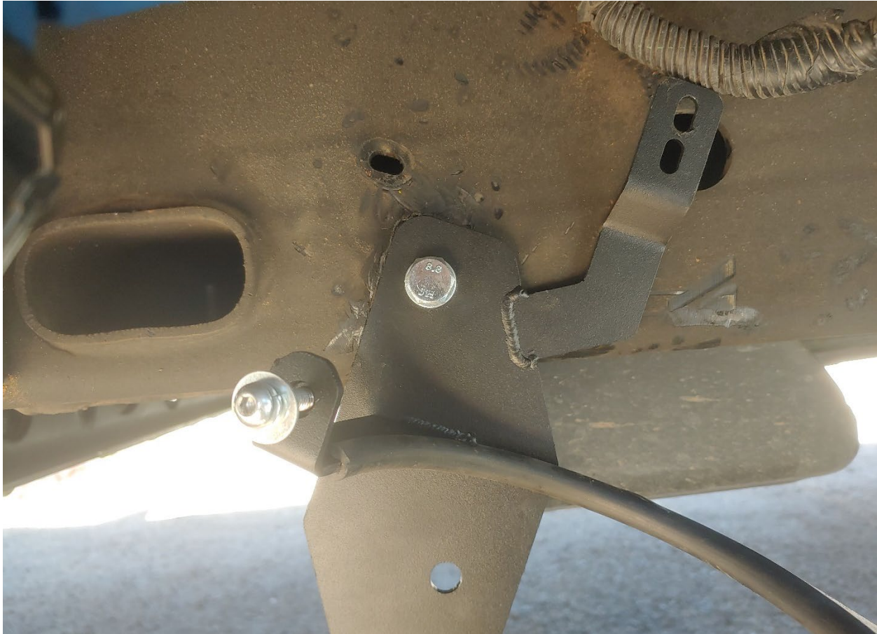
Figure 19- Tank Bracket Installation 1, Diesel
