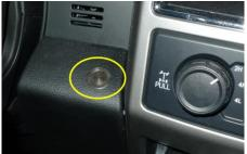
Figure 14: Horn Button Installed in Dash
