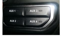
Figure 15: OE Upfitter Switches
