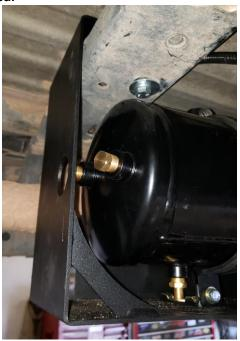
4. Use <u>H7</u>, <u>H9</u>, <u>H10</u>, <u>H11</u>, <u>H21</u>, & <u>C4</u> to secure the back of the compressor mounting plate to the front crossmember. Use any hole in crossmember that is accessible. (<u>C4</u> not shown)
