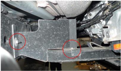
Figure 11: Splash Shield Mounting Points
