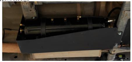
2. Use 2x H4, H5, & H6 to secure the front of the bracket to the skid plate (1).
