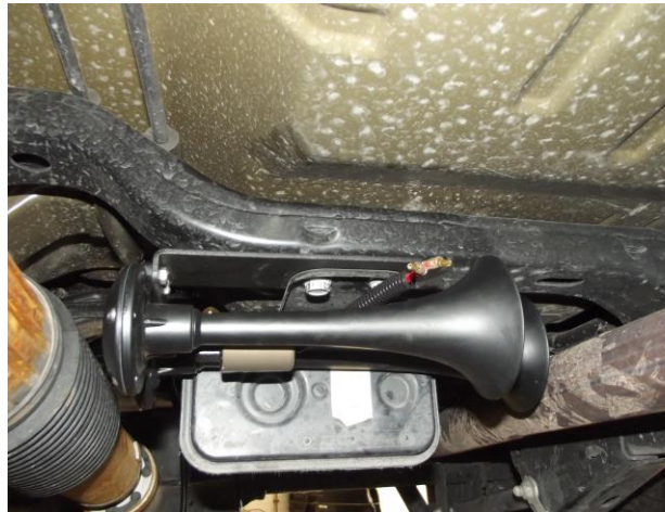
Photo 10 – Air horn bracket mounted under EVAP unit bracket
