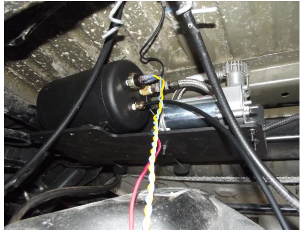
Photo 8 – Air tank positioned on mounting bracket. Note how the braided steel leader hose is looped between the compressor body and the mounting bracket. (NOTE: Tank shown is a previous model. See Photo 8a for new model port connections. Physical location remains the same.)
