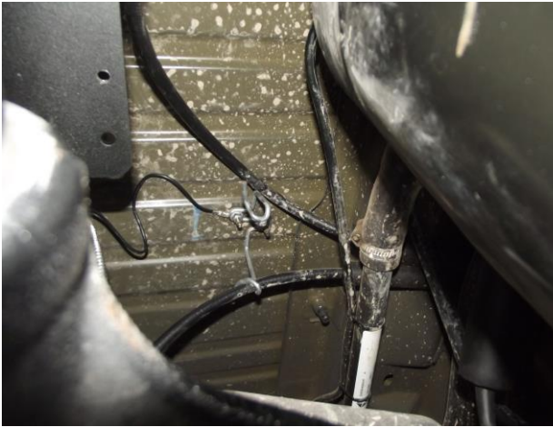
Photo 7 – Emergency brake cable support
