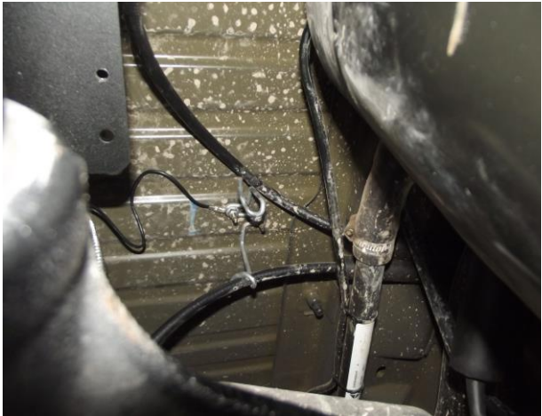
Photo 7 – Emergency brake cable support
