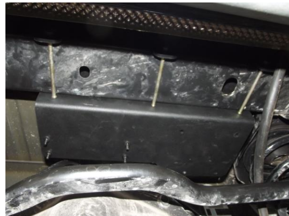
Photo 6 – Mounting bracket, as seen from underneath.
