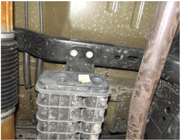
Photo 9 – EVAP canister. Note the two 5/8” mounting bolts
