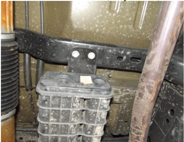
Photo 9 – EVAP canister. Note the two 5/8" mounting bolts
