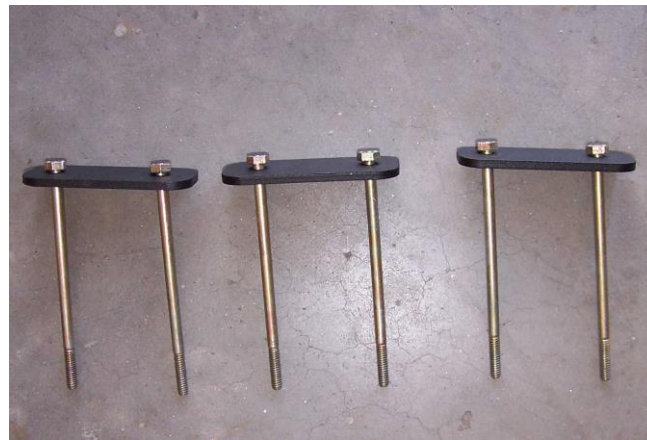
Photo 2 – Rear Mount Plates with bolts inserted
