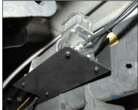
Image D - Compressor Location on Bracket with remote intake air line installed
