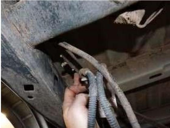
Image G – Separate wiring harness from frame
