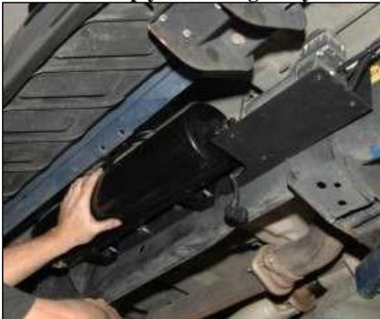
Image C - Air Tank Location on Frame
