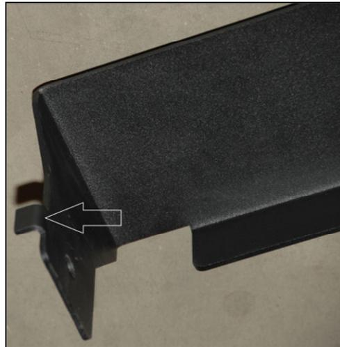
*Image J– Horn Mounting Bracket stabilizing tab*
