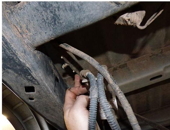
Image G – Separate wiring harness from frame
