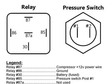
Pressure Switch Post #2..... Switched (on/off with key) +12v
